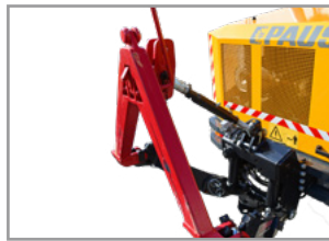
Two double-acting lifting cylinders, mechanical top link
