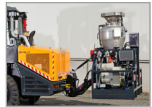
ANFO tank and compressor mounted on a frame
