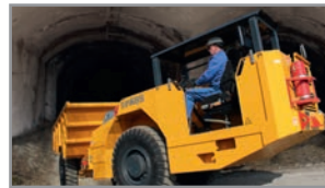
Driver's Seat rotates 180°
