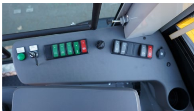
Clearly laid out control panel: The number of switches has been reduced.
