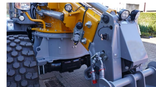
Options: socket, hydraulic oil level check, integrated weighing system, tipping assistant, oscillating axle lock and much more.
