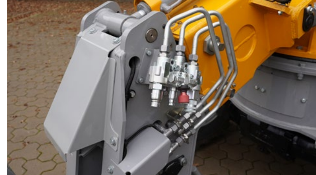
Standard 65 l/min flow in the first auxiliary circuit for a variety of attachments including pressure relief as standard.
