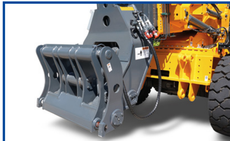
Paus Quick Attachment System with automatic locking
