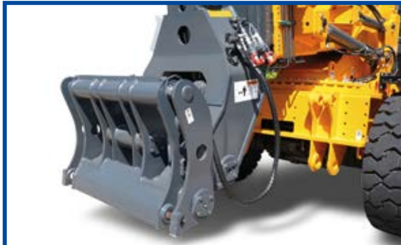
Paus Quick Attachment System with automatic locking
